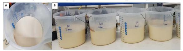
Figure 2: Tests of Biodetergent production to evaluate physical parameters for the volume of 6 liters. (A) aspect of the formulation right after production. (B) production tests for some investigated stirring times
