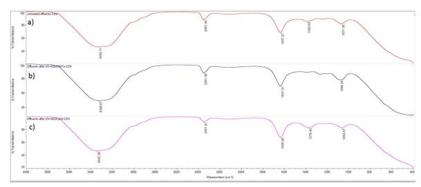
Figure 1: FT-IR analysis of (a) untreated effluents, (b) effluents after UV/K<sub>2</sub>S<sub>2</sub>O<sub>8</sub>/Fe(II) and (c) effluents after UV/H<sub>2</sub>O<sub>2</sub> at pH 3
