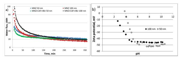
Figure 4: (a) Water flux during the membrane filtration (b) Zeta potential of the membrane with pore size of 50 nm and 100 nm at 1 mM KCl.
