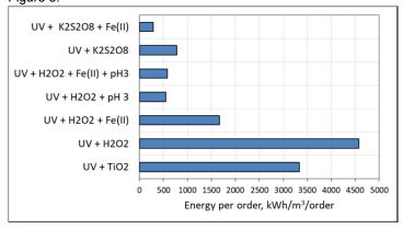
Figure 3: Energy per order for photochemical treatment of MNZ containing effluents
