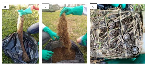
Figure 2: a) Reactor being disassembled during sample collection periods (1, 84 and 168 days) with details of the intense root formation; b) Amount of biomix recovered and sent to the laboratory; c) Detail of the colonization of lignolytic fungi (white rot fungi).
