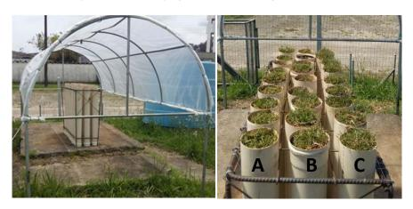
Figure 1: Test condition of columnar field reactors with grass cover detail, being row "A" reactors without contamination, row "B" reactors with contamination of pre-treated effluent and row "C" reactors with contamination of effluent without pre-treatment. Photo: The authors
