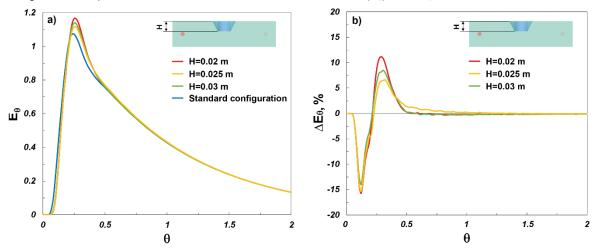
Figure 3. Normalized residence time distributions ( $E_{\theta}$ ) and  $\Delta E_{\theta}$ % for investigated chamber configurations.
