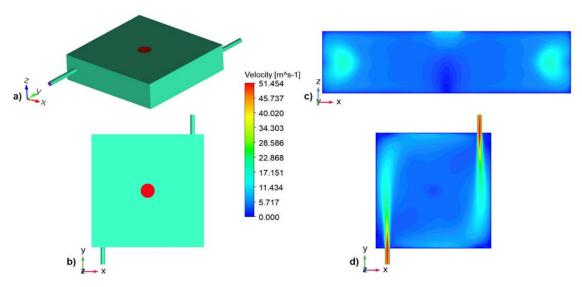
Figure 1. Geometry (a-b) and velocity field (c-d) of the "standard" cyclonic combustion chamber.
