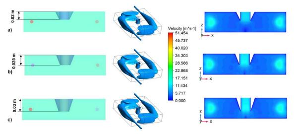
Figure 2. Combustion chamber configuration, iso-surfaces at v=6 m/s and velocity field on the xz plane for three different protrusion lengths: a) 0.02 m; b) 0.025 m; c) 0.03 m.
