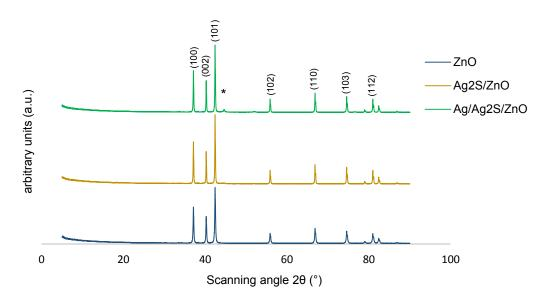
Figure 1: XRD pattern of crystalline ZnO, Ag<sub>2</sub>S/ZnO and Ag/Ag<sub>2</sub>S/ZnO
