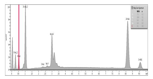
Figure 3: EDX spectra of ternary Ag/Ag<sub>2</sub>S/ZnO nanopowder.
