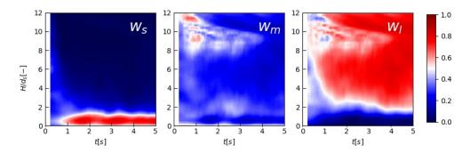
Figure 3: Experimental measurements of small (on the left), medium (in the middle) and large (on the right) particles in time and throughout the dimensionless depth of the flowing layer (i.e.  $H/d_s$ ). The mixture under analysis is mixture 1, which is characterized by  $w_s = 20\%$ ,  $w_M = 30\%$  and  $w_L = 50\%$ .
