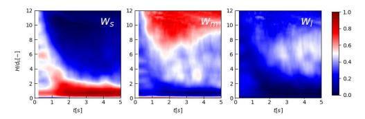
Figure 4: Experimental measurements of small (on the left), medium (in the middle) and large (on the right) particles in time and throughout the dimensionless depth of the flowing layer. The mixture under analysis is mixture 5, which is characterized by  $w_{\rm S}=40\%$ ,  $w_{\rm M}=40\%$  and  $w_{\rm L}=20\%$ .
