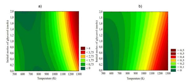
Figure 1: Hydrogen formation along the glycerol SCWG using Gibbs energy minimization methodologies (a) and entropy maximization (b)
