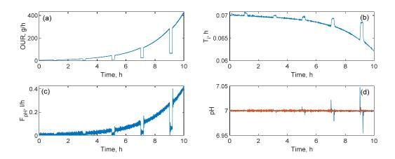
Figure 4: Adaptive control system output: (a) time profile of OUR, (b) adaptation of  $T_i$  controller parameter, (c) feeding solution rate (control variable), (d) comparison of the adaptive (–) and standard (–) PI controller performance
