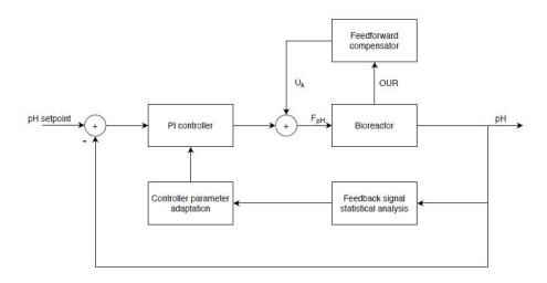
Figure 3: Block-diagram of the adaptive pH control system
