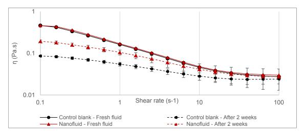
Figure 6: Rheological behaviour of nanofluids and control blank freshly prepared and after 2 weeks
