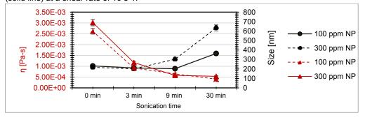
Figure 4: Viscosity at 10 s -1 and particle size of NP suspensions as a function of sonication duration. Left axis: viscosity η (red); Right axis: nanoparticles size (black).
