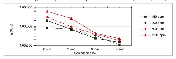
Figure 1: Effect of sonication on viscosity curves for xanthan gum solutions at a shear rate of 10 s-1
