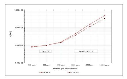
Figure 3: Dilution curve of xanthan gum with 3% NaCl. Shear rates of 6.31 s-1 and 10 s-1.
