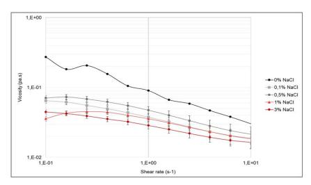
Figure 2: Effect of NaCl on the rheology for xanthan gum solutions.
