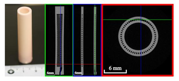
Figure 4. a) Picture of heat exchanger after sintering (left). b) MicroCT scan of heat exchanger -scanned at 70 kV, 141 uA- (middle to right).
