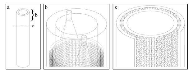
Figure 2. CAD Model of heat exchanger a) Outer appearance of heat exchanger (left). b) Flow distributor (middle). c) Staggered microcolumns array – lid and top cut for clarity – (right)
