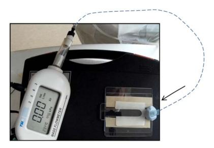
Figure 3: The basic video frame captured during the measurement. The dashed line shows schematically the hose for air delivery to the channel.
