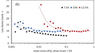
Figure 4: (a) the apparent viscosity and (b) the loss factor measured during frequency sweep of tested non-Newtonian liquids (concentrations of CMC+MIC aqueous suspension shown in the figures).
