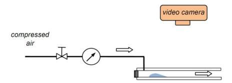
Figure 2: Experimental set-up for liquid displacement in a shallow channel.
