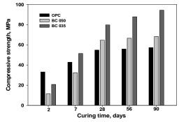
Figure 1: Results of compressive strength measurements for OPC, BC 050 and BC 035 at various curing periods.
