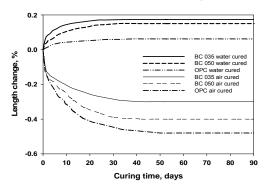
Figure 2: Dimensional stability curves for OPC, BC 050, and BC 035 (air and water cured).
