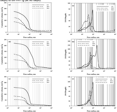
trend, being bimodal for BC 050, and unimodal for BC 035 (Figures 5a, 5b, and 5c right). Moreover, as curing time increases, the cumulative pore volume of the OPC system reduces, passing from about 175 mm<sup>3</sup>/g (at 2 days) to 89 mm<sup>3</sup>/g (at 90 days).
