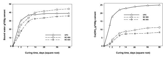
Figure 4: Bound water (left) and calcium hydroxide concentration (right) from TG data (normalized to 100 g of anhydrous cement) vs. curing time for OPC, BC 050 and BC 035.
