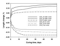
Figure 2: Dimensional stability curves for CSA-based cements (air and water cured).
