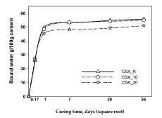
Figure 4. Bound water as determined up to 56 days of hydration (normalized to 100g of anhydrous cement) for CSA\_R, CSA\_10 and CSA\_20 plotted against curing time.
