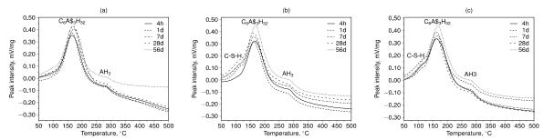
Figure 3: DT results for CSA\_R (a), CSA\_10 (b) and CSA\_20 (c) hydrated for 4 hours, 1, 7, 28 and 56 days. Legend: CaO·Si $O_2$ ·H<sub>2</sub>O=C-S-H; 3CaO·Al<sub>2</sub> $O_3$ ·3CaSO<sub>4</sub>·32H<sub>2</sub>O=C<sub>6</sub>A\$<sub>3</sub>H<sub>32</sub>; AH<sub>3</sub>=Al<sub>2</sub> $O_3$ ·3H<sub>2</sub>O.
