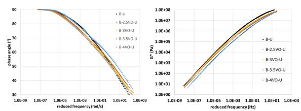
Figure 5 Phase angle (left) and magnitude of complex modulus (right) master curves of the unaged original and rejuvenated binders.
