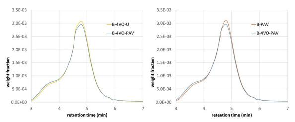
Figure 2: GPC curves of binder B-4VO before and after PAV aging (left); comparison of binders B-PAV and B-4VO-PAV (right).
