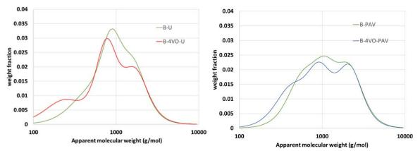
Figure 4: Comparison of the AMWD of the original binder and of the rejuvenated binder (left) and of the binder at the end of the first and second simulated life cycle (right).
