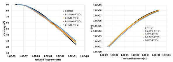
Figure 6 Phase angle (left) and magnitude of complex modulus (right) master curves of the RTFO aged original and rejuvenated binders.
