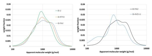
Figure 3: AMWD of the original binder at different levels of aging (left) and comparison of the distributions before and after addition of RJ (right).
