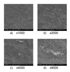
Figure 1: Microstructure of Cu-Cr-Zr sample - General aspect
