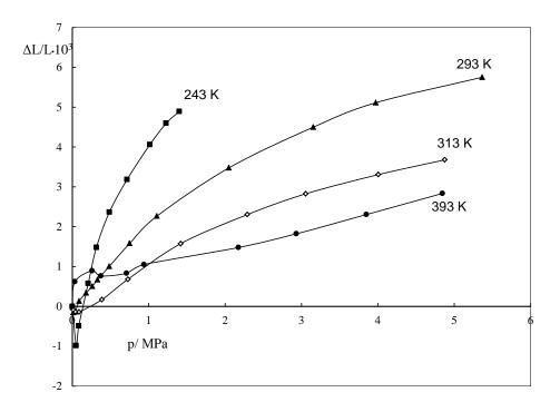
Figure 3: Dependencies of relative linear adsorbent deformation  $\Delta L/L$  on p at different temperatures (adsorptive - CO<sub>2</sub>).
