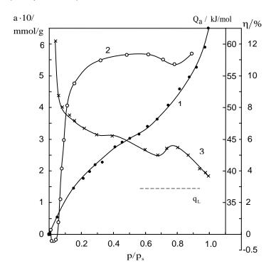
Figure 4: Na- montmorillonite/methanol vapor system: Isotherm (1), dilatometric curve (2) and differential calorimetric heat  $Q_a$  as a function of  $p/p_s$  value (3). Temperature of experiment was 293 K.
