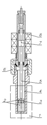
Figure 2: Dilatometric part of the unit: 1, thermostat; 2, quartz polished disks; 3, adsorbent; 4, ampoule with the adsorbent; 5, rod; 6, nut; 7, core; 8, transformer (Tvardovskiy et all. 2011)
