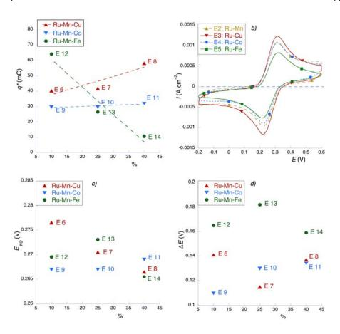
Figure 2: (a) Effect of the third element nominal percentage on voltammetric charge recorded at 10 mV·s<sup>-1</sup> in the range 0.0-1.0 V in Na<sub>2</sub>SO<sub>4</sub>=0.5 M; (b) Cyclic voltammograms for binary films in the presence of the  $Fe(CN)_6^{3-/4-}$  couple; (c) Formal electrode potential measured (d) Anodic-to-cathodic peak separation. Conditions for b), c) and d) are: 0.01 M  $Fe(CN)_6^{3-/4-}$ , 50 mV·s<sup>-1</sup>.
