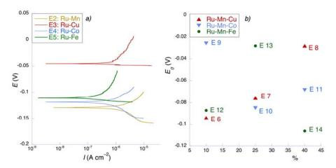
Figure 3: Potentiodynamic polarization curves for binary electrodes (a); Effect of the third element nominal percentage on the Corrosion Potential,  $E_0$  (b). Conditions: Na<sub>2</sub>SO<sub>4</sub>=0.5 M, v=0.1 mV·s<sup>-1</sup>.
