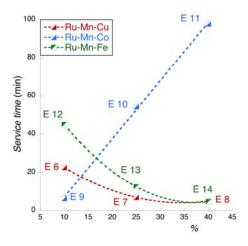
Figure 4: Effect of the composition on the stability of the electrodes expressed as the time required to reach the potential of 7 V. Conditions: Sel 1 cm<sup>2</sup>; Ref. Ag/AgCl; j= 4000 A·m<sup>-2</sup>; V = 50 ml H<sub>2</sub>SO<sub>4</sub> 0.5 M, T=28±0.5 °C; mix = 500 rpm
