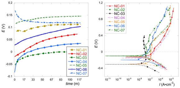
Figure 2: (a) Open circuit potential (OCP) curves; (b) Potentiodynamic polarization curves. Conditions:  $Na_2SO_4=0.1 M$ ,  $v=0.1 mV \cdot s^{-1}$
