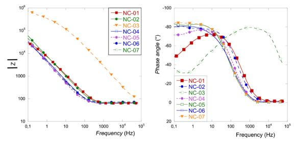
Figure 3: Electrochemical impedance Bode plots for (a) impedance magnitude (|Z|); (b) phase angle ( $\theta$ ) vs. frequency (f). Conditions: Na<sub>2</sub>SO<sub>4</sub>=0.1 M.
