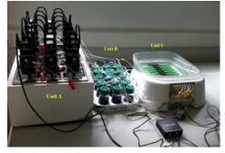
Figure. 1: Automatic methane potential test system (AMPTSII) (Browne, 2013)
