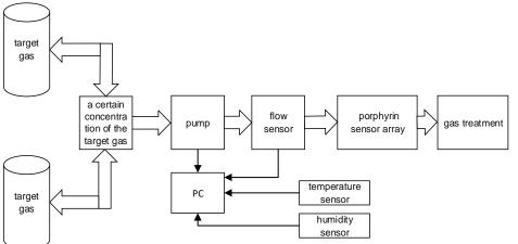
Figure 1: Schematic diagram of porphyrin sensor detection system
