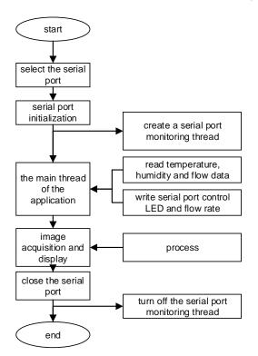
Figure 3: Diagram of serial communication
