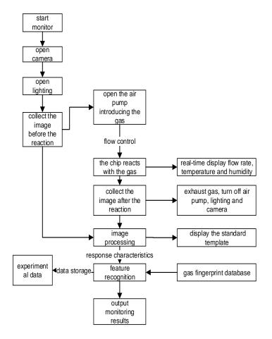
Figure 2: Schematic figure of gas detection system
