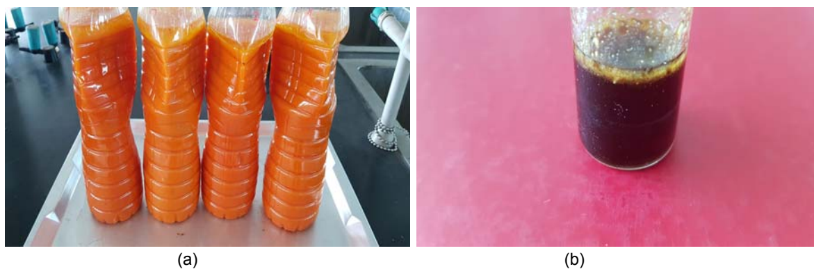
Figure 5: Photo of (a) CPO after methanol extraction and of (b) oil residue after methyl ester evaporation
