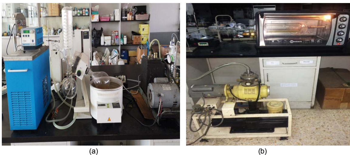
Figure 1: Photo of (a) Buchi rotary evaporator and of (b) in-house Kugelrohr distillation apparatus set
