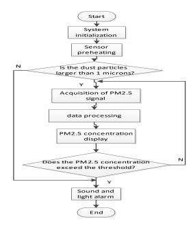
Figure 5: System software design flow
