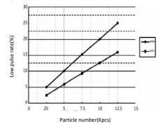
Figure 2: The relationship between the low pulse rate and the number of particles
