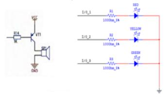
Figure 4: Sound and light alarm indicator circuit
