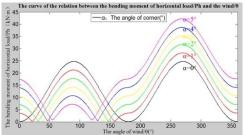
Figure 4: The relationship among wind angle, wire angle and horizontal force
