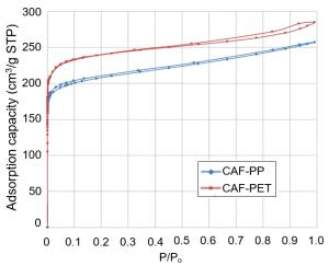
Figure 5: Adsorption desorption isotherms of N2 on 2 samples: CAF-PP and CAF-PET
