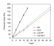
Figure 6: Pressure drop of non-woven fabric (PP, PET) and CAF (CA-PP, CA-PET) with different number of filter layers
