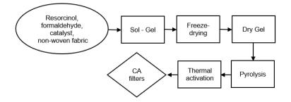
Figure 1: The process of synthesizing carbon aerogel filters
