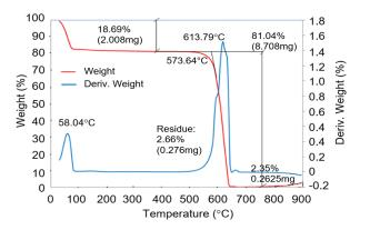
Figure 3: Thermogravimetric analysis (TGA) results for CAF
