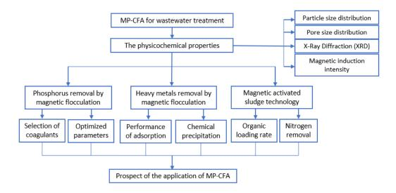
Figure 1: Outline of the procedures for the application of MP-CFA to wastewater treatment.
