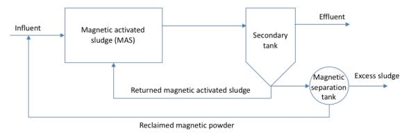
Figure 2: Diagram of magnetic activated sludge (MAS) process
