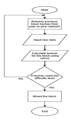
Figure 2: Flowchart of the mining process.
