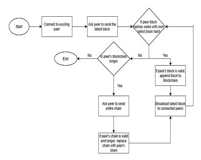
Figure 3: Communication between nodes.
