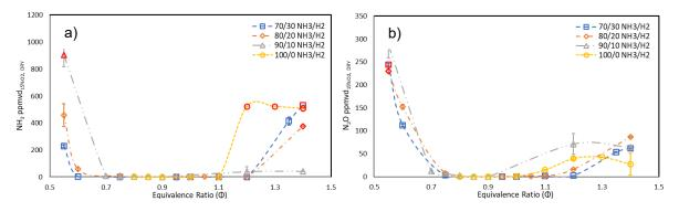
Figure 3:  $NH_3$  emissions (a), and  $N_2O$  emissions (b) for all blends and equivalence ratios. Red coloured symbols are out of the measurement range.
