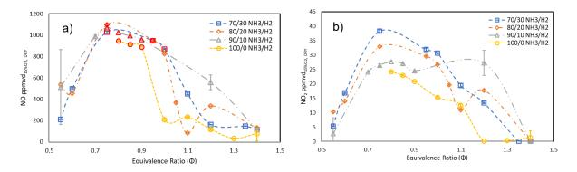
Figure 2: (a) NO emissions, and (b) NO<sub>2</sub> emissions for all blends and equivalence ratios. Red coloured symbols are out of the measurement range.
