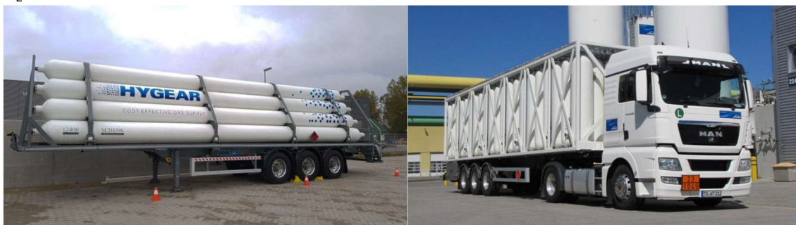
Figure 1: A tube trailer and composite cylinders battery pack as operated by Linde gas
