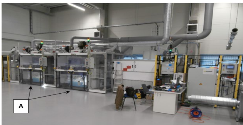
Figure 2: High-capacity production line for continuous production of nanofibre textiles of Nano Medical s.r.o. The letter A indicates the location of the spinning units with polymer material containers
