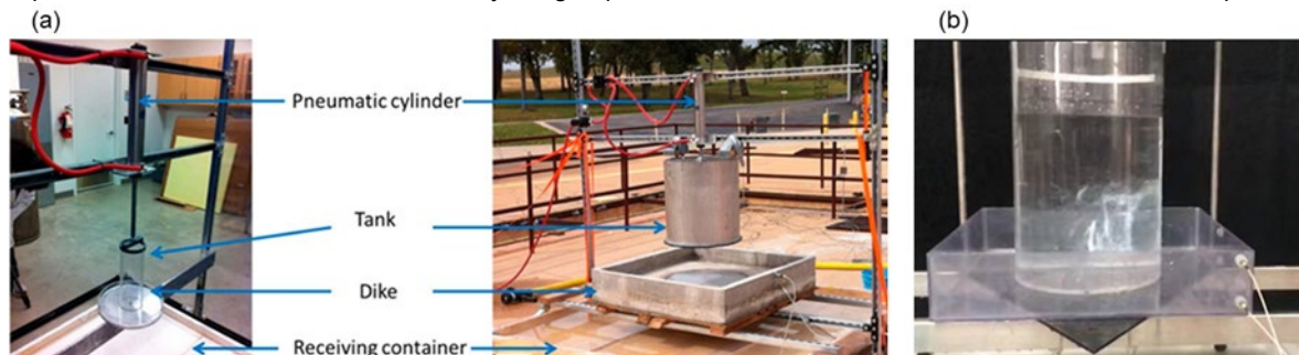
Figure 1. Experimental setups for overtopping (a) (Zhang et al., 2017) and bund with pressure sensors (b)
