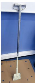
Figure 2: Shovel used for the cleaning operation made of stainless steel and of a bronze plate at the extremity
