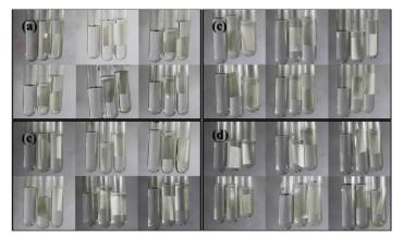
Figure 2: Three samples of each type of solution of Ferrous Ammonium Sulfate, Potassium Dichromate, Cadmium Sulfate, and Lead Nitrate were run. These solutions contain the heavy metals Fe, Cr, Cd, and Pd, respectively, with an increasing concentration of 0.05 ppm to 1.0 ppm. The left-most solution served as the control (no paper strip), while the second and the third samples contained a paper strip coated with kalachuchi latex to detect the presence of heavy metal ions present in each solution.
