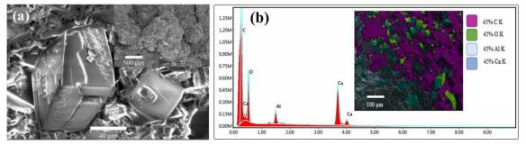
Figure 1: (a) SEM image of the dried and pulverized latex sample and (b) elemental mapping by EDX analysis
