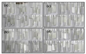
Figure 4: Test tubes showing solutions of (a) Ferrous Ammonium Sulfate (b) Potassium Dichromate (c) Cadmium Sulfate (d) Lead Nitrate with increasing concentrations (0.05, 0.1, 0.25, 0.5, 0.75, 1 ppm) respectively. Paper strips used came from a paper sheet coated with 5 ml of latex. Each test included a control (solution without paper strip) and two replicates for each concentration.
