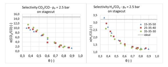
Figure 3: Selectivity for  $H_2/CO_2$  and  $CO_2/CO$  on stagecut for the three mixtures with permeate pressure  $p_P = 2.5$  bar on stagecut.
