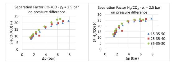
Figure 5: Separation factors on total pressure drop for three different mixtures.
