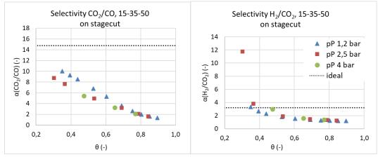
Figure 2: Selectivity for H<sub>2</sub>/CO<sub>2</sub> and CO<sub>2</sub>/CO on stagecut for mixture 15-35-50 on stagecut.
