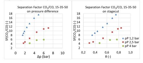
Figure 4: Separation factors CO<sub>2</sub>/CO for three permeate pressures on pressure difference and stagecut.
