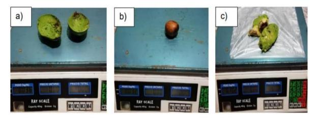
Figure 1: Weighing of avocado components: a) Mass of avocado peel, b) Mass of avocado pit and c) Mass of avocado pulp
