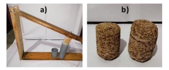
Figure 2: Production of ecological briquettes: a) Manual briquetting press and b) Ecological briquettes
