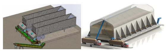
Figure 1. Examples of horizontal silos (BE&E, 2016).
