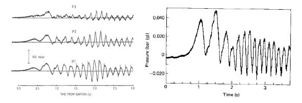
Figure 4. Left: Oscillatory pressure development resulted in the ignition of the upper half of a silo of 236m<sup>3</sup>. The fuel is cornstarch 600g/m<sup>3</sup> and vented on the roof with 5,7m<sup>2</sup> vents. Right: Pressure vs time measured at 3m above the bottom of the silo. Figure as seen in Eckhoff (2003), Eckhoff (1988) and Eckhoff (1984).
