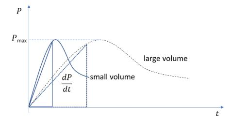
Figure 3. Diagram of pressure vs time showing the difference in rate of pressure and explosion duration for two different volumes; the larger volume is represented by the dashed line.
