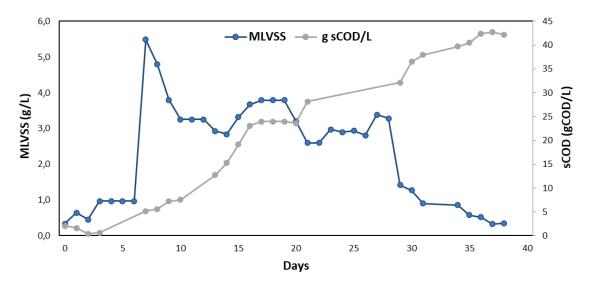
Figure 2. Biomass growth and sCOD of the mixed liquor during the 38 days of the CSTR operation.
