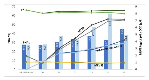
Figure 4. PHAs accumulation test performed with the biomass extracted from the CSTR. The data show the results for the flasks fed with either synthetic VFAs medium (dark shades) or with fermentation fluid (light shades).
