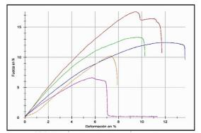
Figure 8: Tensile strength and elongation of sorbets based on Vitis vinifera peel
