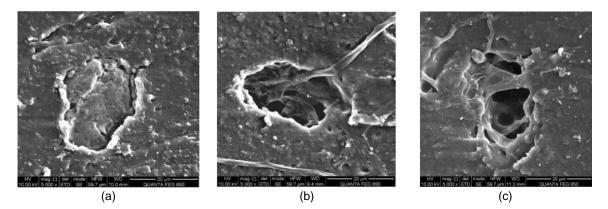
Figure 1: Electron microscopy analysis for the rubber surface (a) before biodegradation and after (b) 16 and (c) 40 days of enzymatic action of the fungus.
