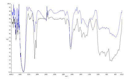
Figure 2: FTIR spectra of rubber samples before inoculation with fungi (black spectrum) and after 45 days of biodegradation (blue spectrum)
