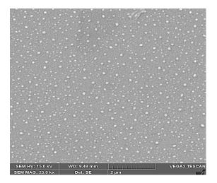
Figure 3: Scanning electron micrograph (25,000 x) of nanocapsules obtained with the parameters described in table 1
