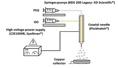
Figure 1: Coaxial electrospray assembly
