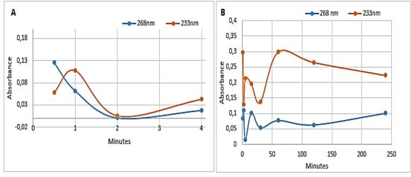
Figure 7: UV-VIS spectroscopy showing the release profile of the nanocapsules (A) in artificial saliva and (B) in a solution similar to body fluids
