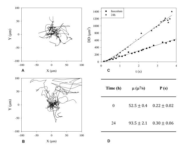
Figure 2: Bacterial trajectory analysis and mean squared displacements. A comparison between inoculum cell trajectories in static condition (A) and 24 hours flux condition (B). To quantitatively assess cell movement, the mean squared displacements vs t data are fit (C) according to eq. 3 obtaining motility parameters reported in the table (D) at inoculum condition and 24h of flow.
