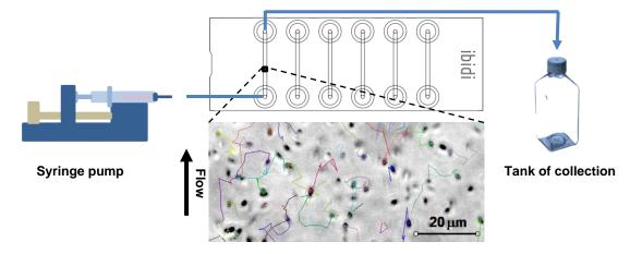
Figure 1: Schematic representation of time-lapse workstation along with an example of bacterial tracking at inoculum condition. Bacterial were identified as a dark object of appropriate dimension ( $2\mu$ m length) on a bright field after image processing.
