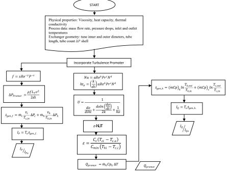
Figure 2: Flow chart of the computation of new thermal and pressure drop of a heat exchanger with turbulence promoters
