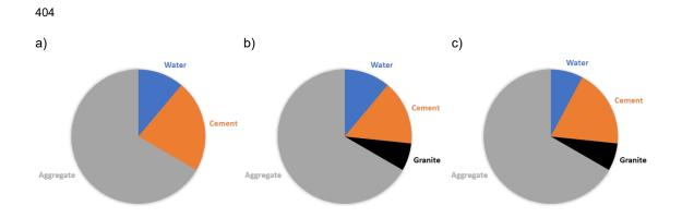
Figure 1: Cementitious composites mixture with: a) ordinary Portland Cement, b) granite powder as a cement substitute, c) granite powder as a cement paste substitute
