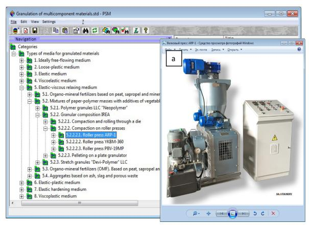
Figure 4: ASRS CALS project: Elastic-viscous medium - Paper-polymer mass - IREA composition - Compaction on roller presses - ARP-1 roller press (a - ARP-1 roller press)
