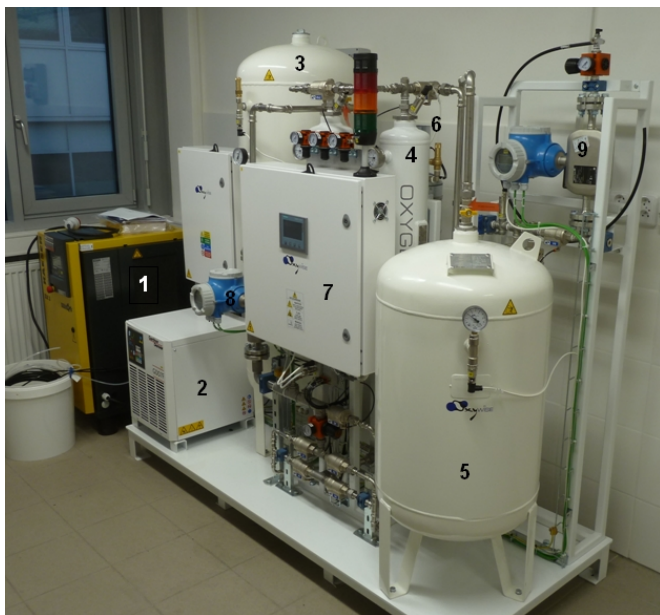
Figure 2: The pilot-plant adsorption unit: 1) compressor, 2) air dryer, 3) air receiver, 4) PSA columns, 5) GOX receiver, 6) exhaust pipe, 7) control unit, 8) mass flowmeter of inlet air, 9) mass flowmeter of product gas
