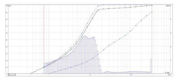
Figure 4: Differential and integral distribution in the composition of a mixture of gypsum binder and ground technogenic basalt powder
