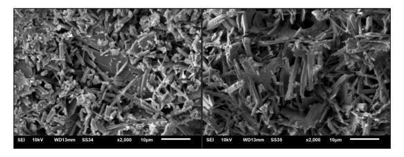
Figure 5: Microstructure of pure gypsum binder (right) and modified with technogenic basalt powder (left)
