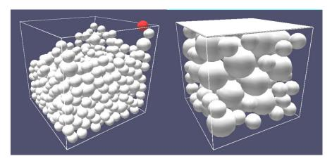
Figure 1: Model of random packing of particles in the system gypsum binder-technogenic basalt powder
