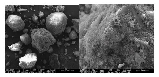
Figure 3: Microstructure of technogenic basalt powder
