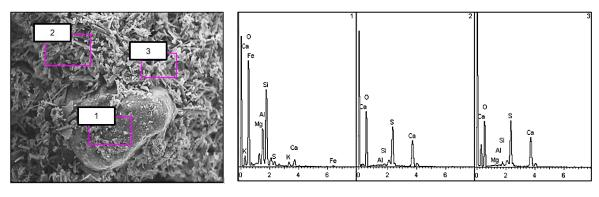
Figure 6: Microstructure of gypsum stone modified with technogenic basalt powder, aluminosilicate ash component and slaked lime and obtained spectra
