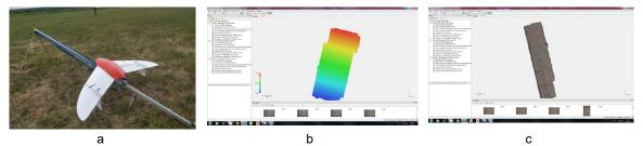
Figure 5: Geoscan 201 Agro UAV data processing in Agisoft Photoscan of field "KH Mayak" LLC: a) Geoscan 201 Agro UAV, b) DEM in the program, c) orthophotomap of the area
