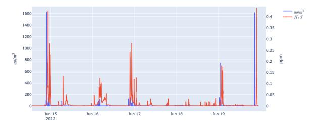
Figure 4 - Values of OU/ m<sup>3</sup> and H<sub>2</sub>S recorded in the period 14 June - 19 June
