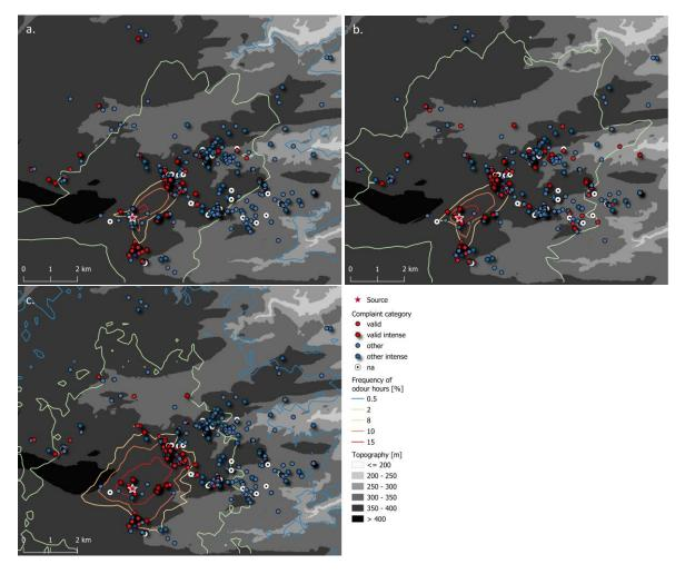
Figure 5: Spatial distribution of complaints categorized according to validity and intensity for (a.) SYMOS, (b.) AUSTAL and (c.) GRAL using  $C_t = 1$  OU<sub>E</sub> m<sup>-3</sup>. Separation distances correspond to the frequency of odour hours.
