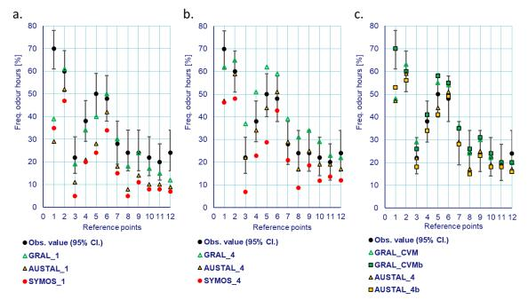
Figure 2: Modelled frequency of odour hours using (a.)  $R_{90} = 1$  and (b.)  $R_{90} = 4$ . (c.) Comparison of Lagrangian models implementing CVM and  $R_{90} = 4$  with the inclusion of buildings (squares).
