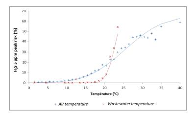
Figure 1: Risk of a 5 ppm H2S peak at SAV depending on air and water temperature
