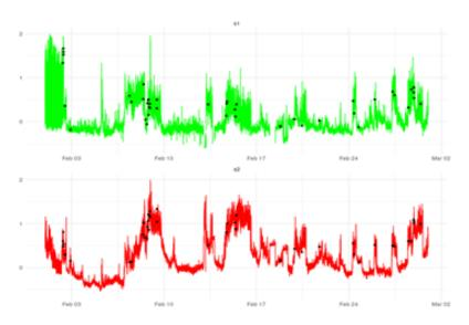
Figure 4: eNoses signals of s1 (green) and s2 (red) channels. Complaints are shown at the related timestamps (black dots).
