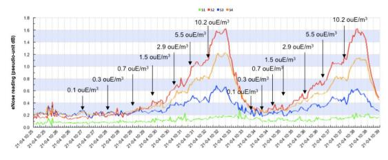
Figure 1: comparison between dynamic olfactometry and eNose readings for the TATA steel sinter plant odour.
